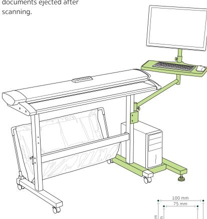
Monitor bracket accepts VESA standard monitors. It has 8 holes arranged in 2 squares: 4 holes at 75 mm and 4 holes at 100 mm measured horizontally and vertically between the centres.
