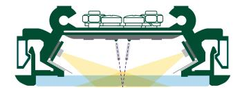
With SingleSensor™ technology, you get an uninterrupted scan line across the full width of the CIS scanner. No stitching or calibration required. The result: quality, convenient scanning.
