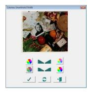
SC TWAIN allows the user to control scan resolution, scan area (paper size), colour mode (RGB, B&W or grayscale), the speed of the scanner and the type of measurement units displayed on the interface. Adjustments to the brightness and contrast of the acquired scan can be viewed and applied via the second screen.
