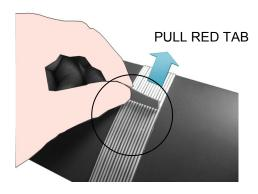
The scanner is protected during shipment by two strips of self adhesive tape which must be removed before proceeding with the installation.
