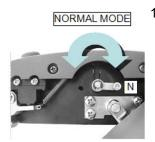
First change the scanner to run in Photo Mode (P) by opening the scanner lid and moving the adjustment lever in the edge of the lid nearest the panel so that it points to the front of the scanner. Loosen the small bolt on the end of the lever before making the adjustment and re-tighten afterwards. Note that the scanner is usually shipped in the Normal (N) Mode (high pressure position).
